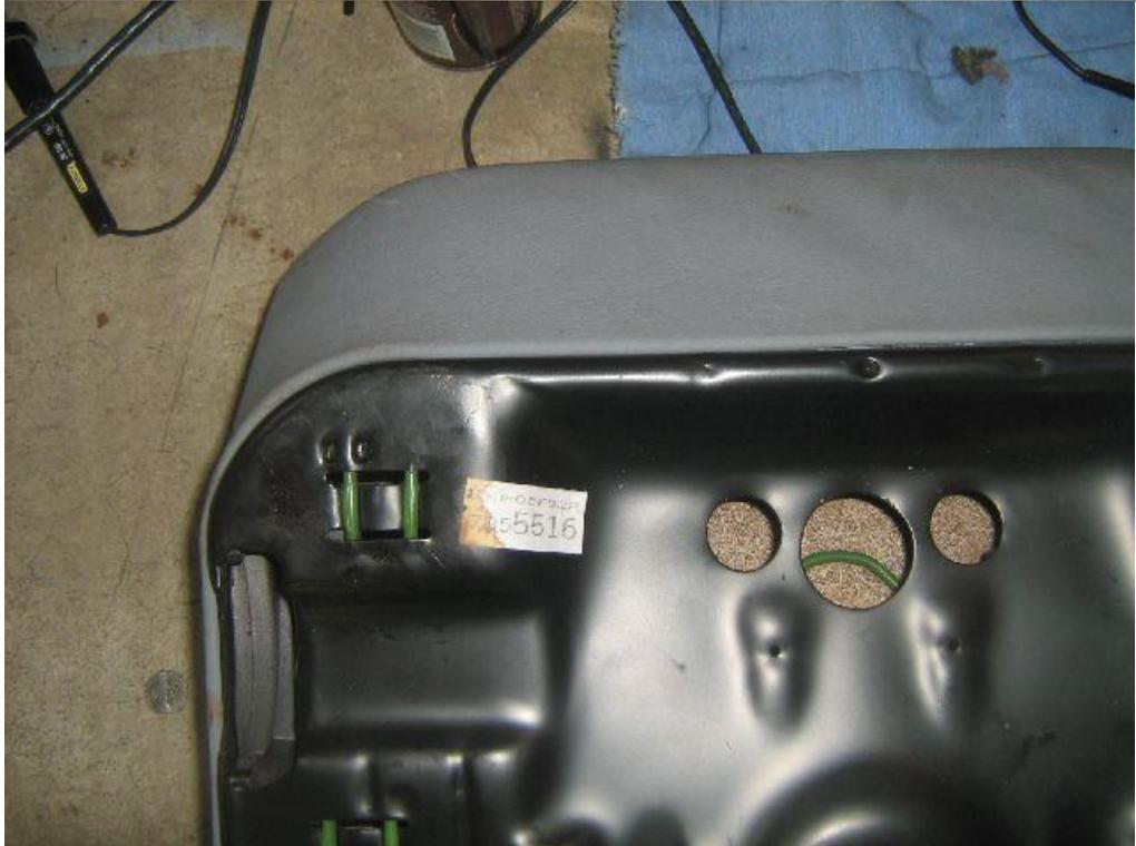
To get to the seat top heater you can remove all of the leather but the most likely place is the left bolster panel so I just removed the back panel and peeled the leather up from the bottom
